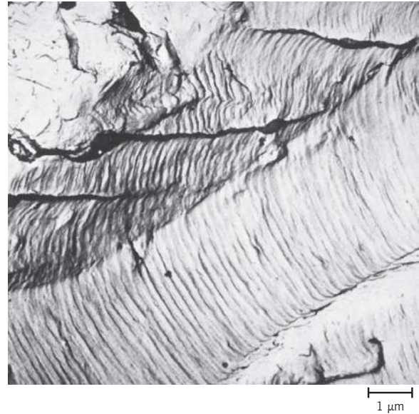
Figure 8.24 Transmission electron fractograph showing fatigue striations in aluminum. 9000X. (From V. J. Colangelo and F. A. Heiser, Analysis of Metallurgical Failures , 2nd edition. Copyright © 1987 by John Wiley & Sons, New York. Reprinted by permission of John Wiley & Sons, Inc.)
