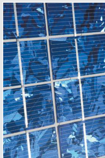
(b) An array of polycrystalline silicon photovoltaic cells.
