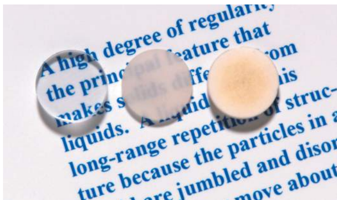
Figure 21.10 The light transmittance of three aluminum oxide specimens. From left to right; single-crystal material (sapphire), which is transparent; a polycrystalline and fully dense (nonporous) material, which is translucent; and a polycrystalline material that contains approximately 5% porosity, which is opaque. (Specimen preparation, P. A. Lessing.)
