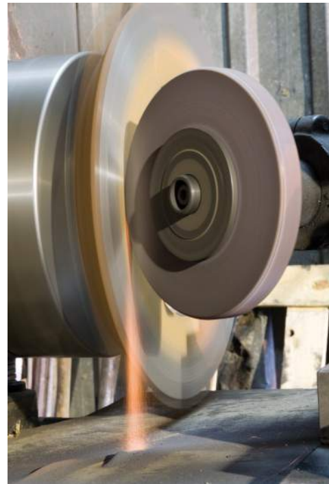
Figure 13.6 Photograph of a clutch lining pressure plate that is being ground with a grinding wheel.
