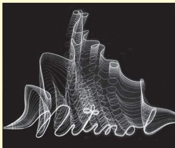
Time-lapse photograph that demonstrates the shape-memory effect. A wire of a shape-memory alloy (Nitinol) has been bent and treated such that its memory shape spells the word Nitinol . The wire is then deformed and, upon heating (by passage of an electric current), springs back to its predeformed shape; this shape recovery process is recorded on the photograph. [Photograph courtesy the Naval Surface Warfare Center (previously the Naval Ordnance Laboratory)].
